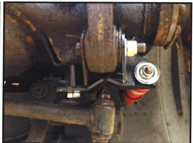
Panhard to axle bolt correct orientation
